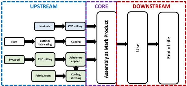
Note: Inputs in white are for both product ranges, inputs in blue are for solid tops, inputs in green for upholstered tops.
